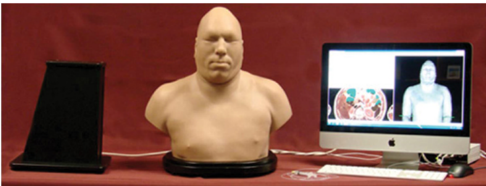
FIGURE 5.7 The rubber bust and skeletal system are built to the geometry of the VH Male. The vertical position of the tip of the “real” needle attached to a “real” syringe (just toward the left of the keyboard) determines which transverse cross section is displayed on the monitor. The syringe and needle are also displayed (updated in real time) on the right-hand side of the monitor. Rotation of the bust rotates the 3D rendering on the monitor. As the user penetrates deep to the skin with the tip of the needle (the entire length of the needle if the syringe and needle are held in a horizontal plane at the correct location of the needle is displayed in the cross section. The needle position can be frozen at any time and the 3D rendering dissected to reveal the entire needle in the 3D VH rendering. An optional display utilizes the orientation of the syringe and needle to control the display of an oblique cross section in place of the transverse cross section. The full length of the needle is always in the oblique cross section.
