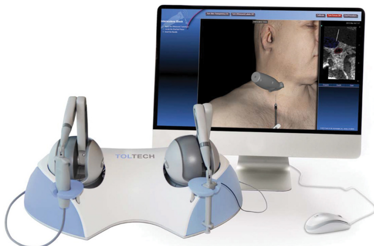
FIGURE 5.8 This virtual reality, partial task trainer is similar to the augmented reality version in Figure 5.7. This trainer includes all the features of the augmented reality version with the addition of ultrasound image guidance training. Haptic response for needle penetration is provided by 3D Systems Omnis. Reproduced with permission of Touch of Life Technologies, Inc.
